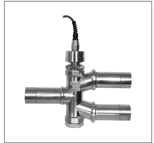
The Sporlan Modulating 3-Way Valves are stepper-motor driven three-way valves for modulation of the two outlet ports and used in such applications as heat reclaim and dehumidification. As port A opens, port B will close and vice versa. Features include:
