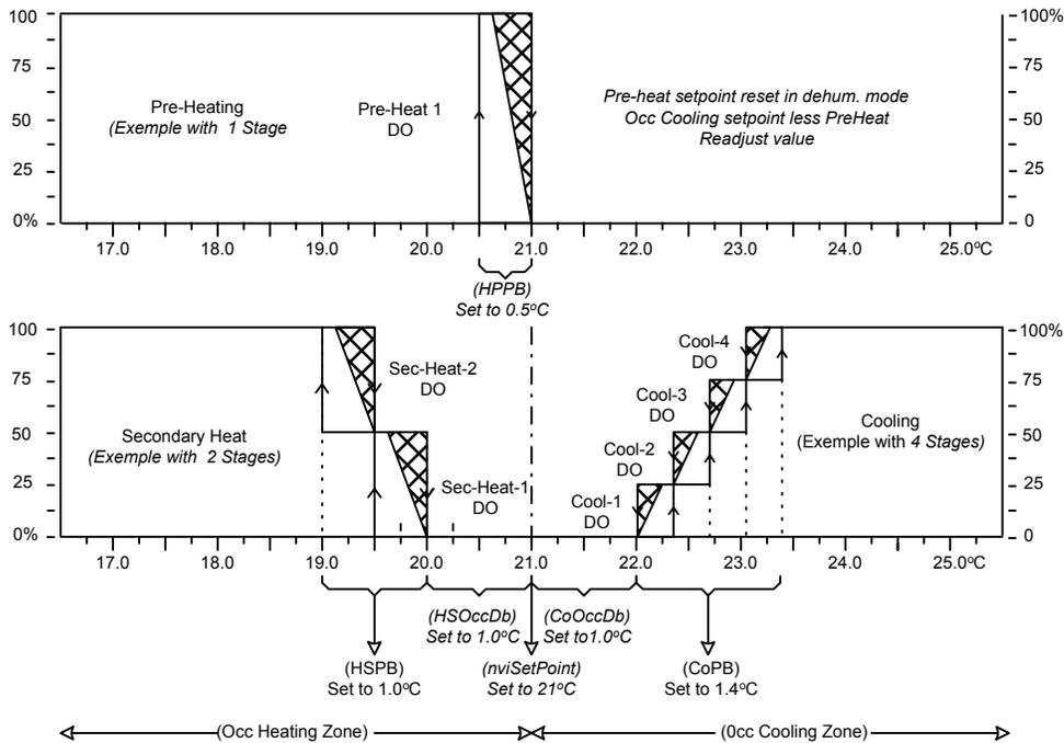
In the figure above the hatched area indicate a modification of the Off trip points due to a hysteresis of 20%.
