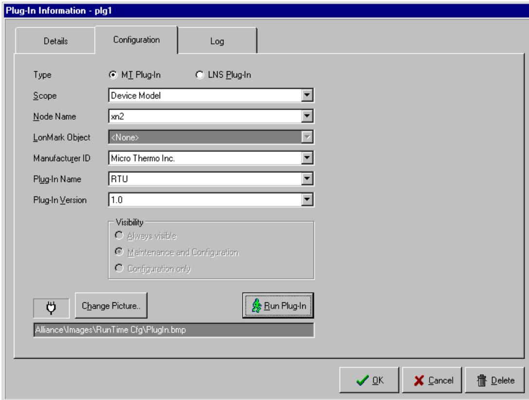
After the plug-in was completely configured, the *Run Plug-In* button allows the technician to start the plug-in.
