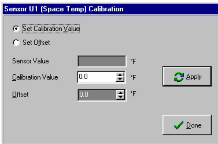
offset so the installer can enter it directly to calibrate the sensor.
