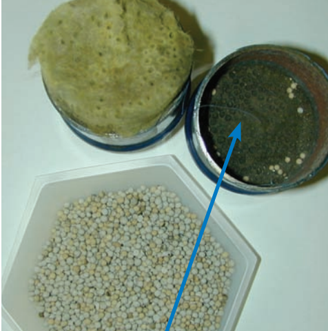
Blockage initiated extreme turbulence in the shell
